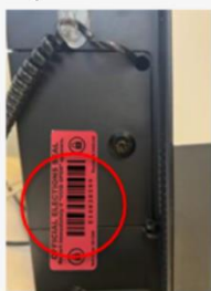
BMD: Two Seals Thumb Drive Compartment Door
